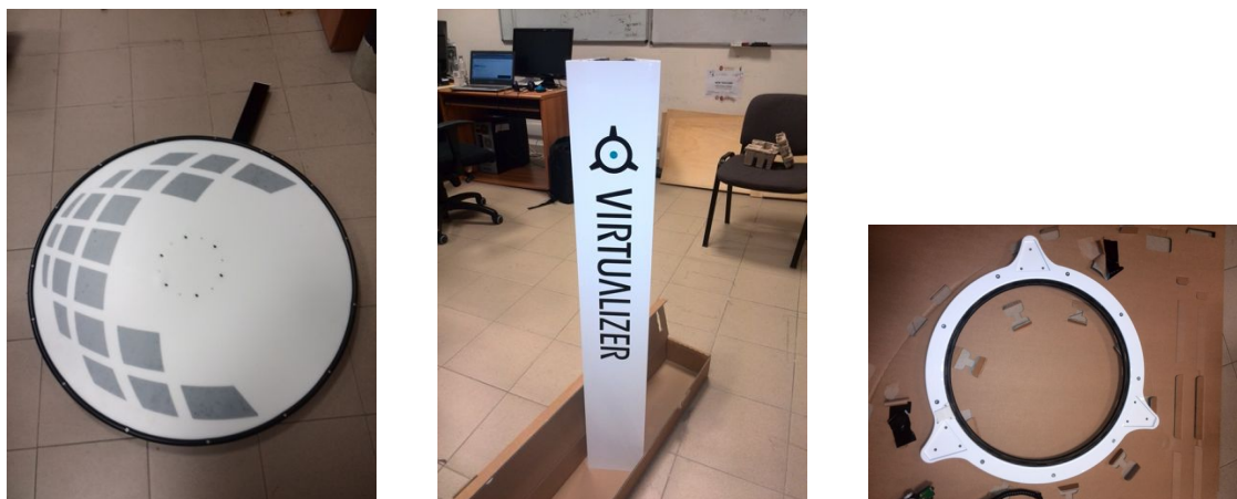
Figure 3: From the right: base plate, pillar and ring-construction
